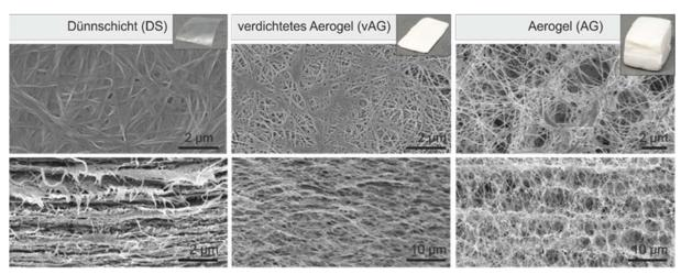
Electron microscopic images of the surface (upper row) and the cross-section (lower row) of the BC membrane types investigated here. In addition, a digital image of the respective membranes is shown, which illustrates their size in the centimeter range.
