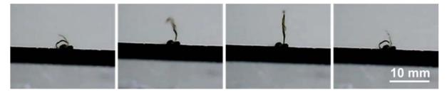
Photographs showing the electrostatic opening of a  $V_2O_5$  scroll: from initial state, applying an electrostatic field by holding the field source above the scroll, fully opened scroll, after removing the field, the scroll returns to its initial state.
