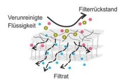
Schematic representation of the project goal, which includes a suitable structuring of cellulose based materials to achieve a multi-stage liquid filtration
